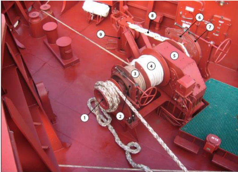
Combined windlass/mooring winch with split drum
